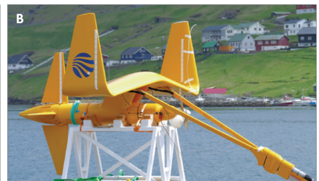
Figure 6: Tidal-kite turbine. (A) Configuration of a tidal kite turbine with schematic flow pattern. Modified after IRENA 2020 (IRENA 2020). (B) One of the 100kW capacity tidal-kites installed on the Faroe Islands (Denmark) (Frangoul 2020).
