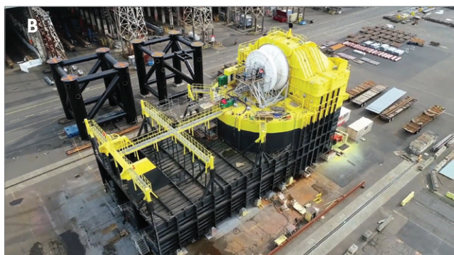
Figure 7: Oscillating water column technology. (A) Configuration of a typical setup. The water surface level changes caused by wave action push air through a wind turbine which works only in one direction. Modified after IRENA 2020 (IRENA 2020). (B) Picture of the OE35 barge, developed by OceanEnergy (Ireland). Submerged parts of the barge are painted black, yellow painted parts are above the water surface (OceanEnergy 2024)
