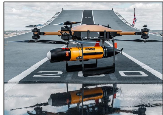
Figure 15. Drone with Autonomous Underwater Vehicle 52
