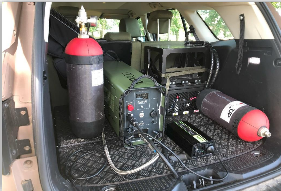
Figure 6: Mobile usage 400W device (NATO ENSEC COE)
