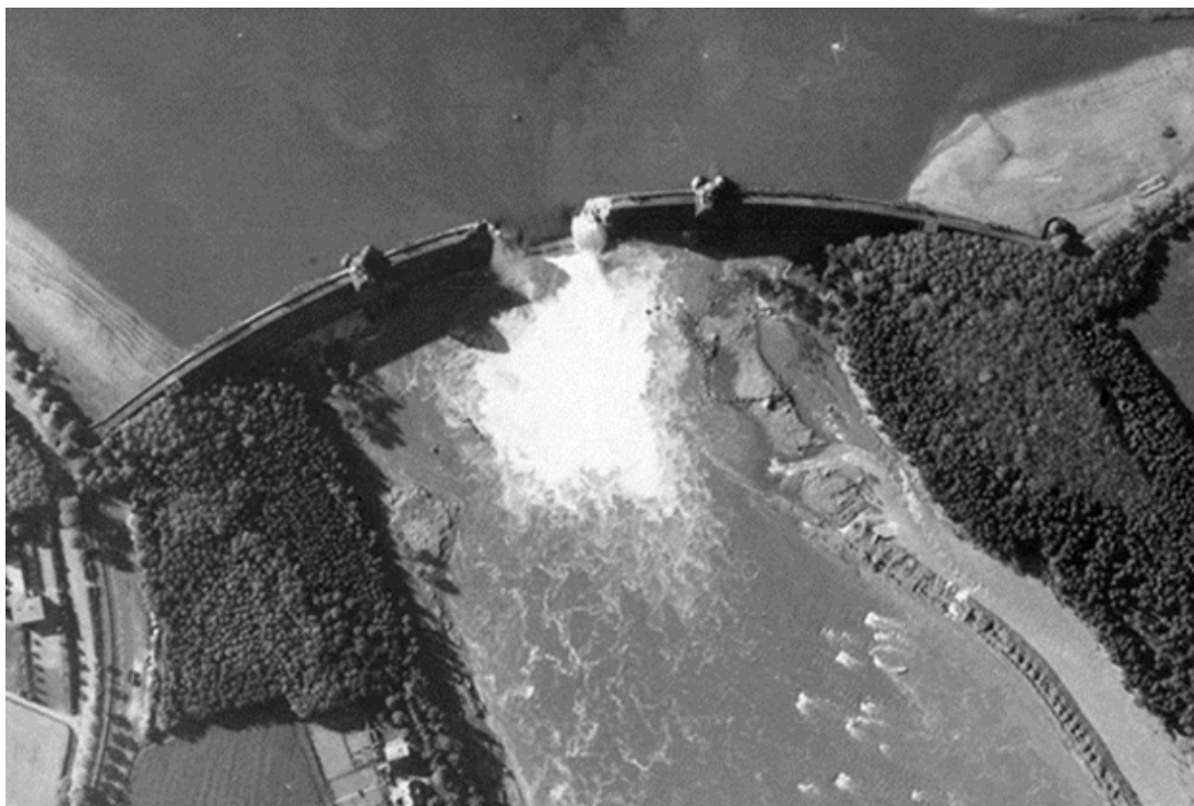
Figure 5 – Aerial photo showing the damage to Mohne Dam, 17th May 1943 (image: NCAP)
