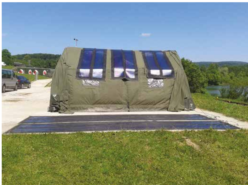
Samples of solar cells on a standard Dutch tent at CL13
