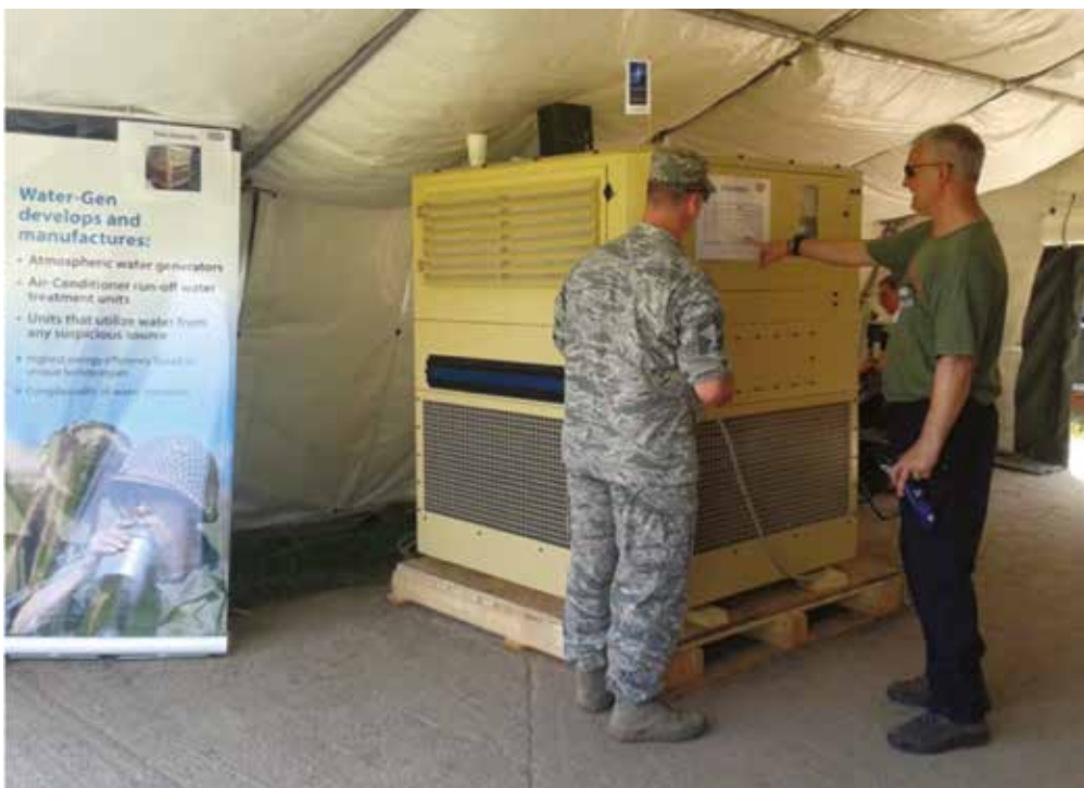
A British representative of the Ministry of Defence demonstrates the atmospheric water generator (a machine taking water out of the air). The machine produced during the CL13 in Slovakia 15 l drinking water per hour using 5 kWh.
