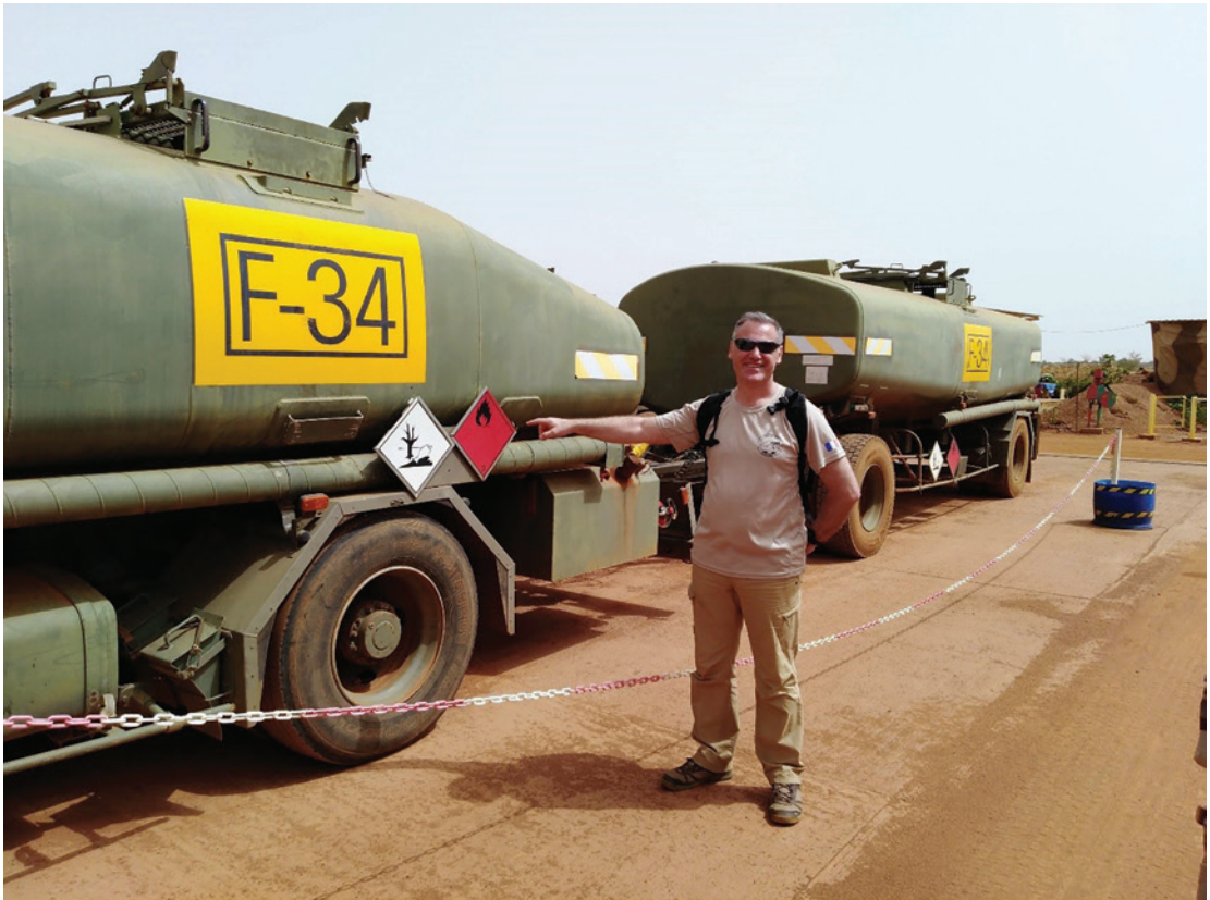
Figure 1: Fuel truck of the French Army Corps d' Essence in a field camp in Niger loaded with NATO F-34 fuel. The fossil carbon based F-34 is currently the standard liquid fuel for military aviation and also the basis of truck diesel in NATO forces (Photo: Zimmermann 2019).
