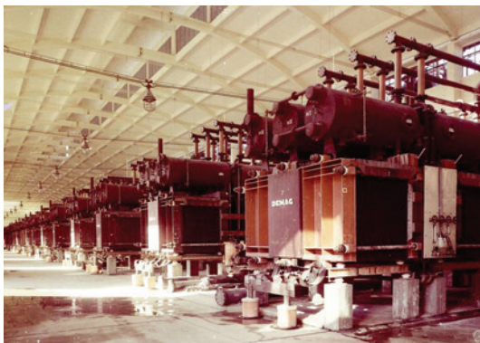
Figure 5: Array of electrolysers in the Aswan hydroelectric dam, Egypt (Hydrochenik 2020). These electrolysers were installed in 1960 and were mainly used for providing hydrogen for nitrogen based fertilizer production.
