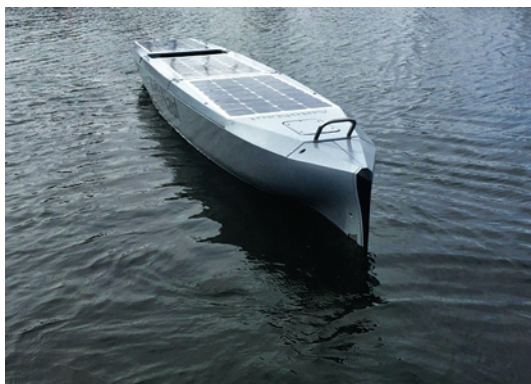
AutoNaut is a marine drone for ocean surveillance, partially printed in 3D and which function by wave energy and solar panels.
