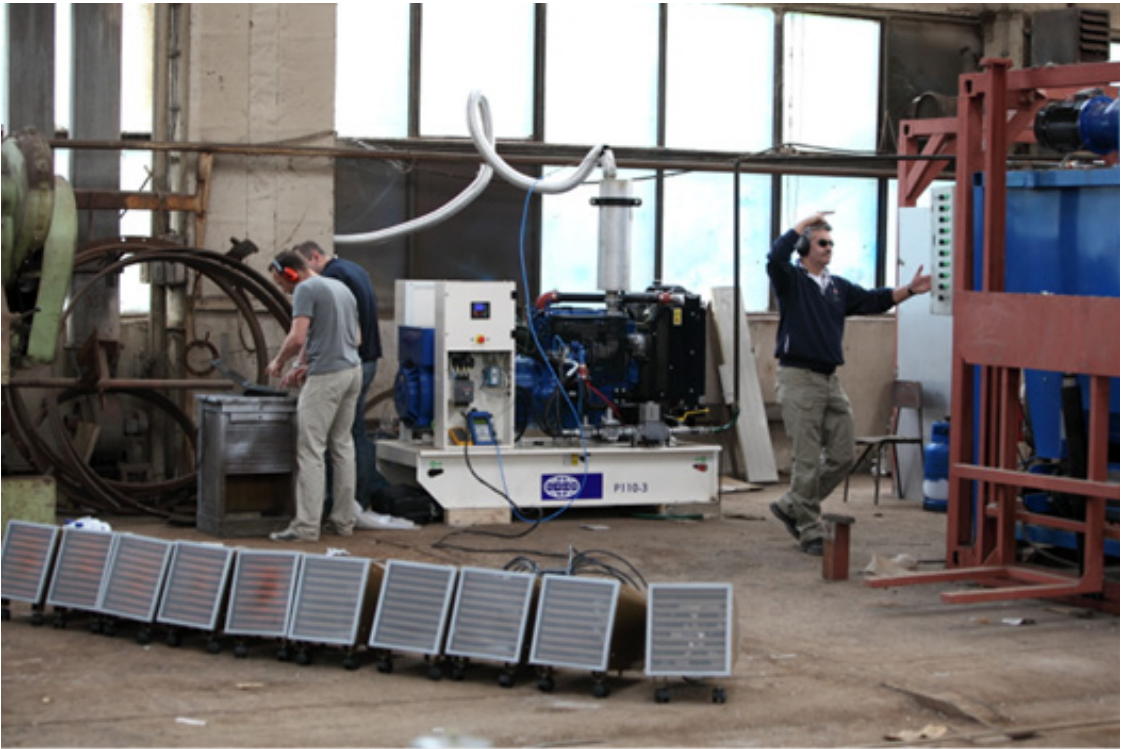
Figure 4 Testing WER with diesel generator
