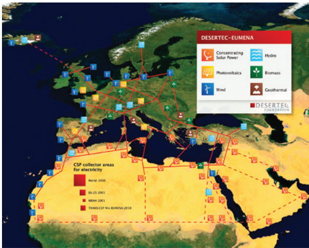
Figure 5: Concept of a transcontinental power grid supplied by renewable energy proposed by the DeserTEC Foundation in 2009 12 .
