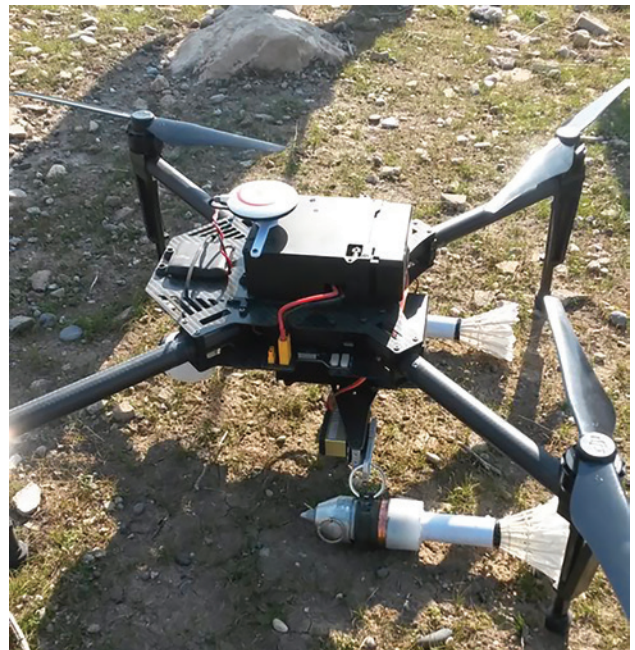
Figure 9. Drone with ordnance and camera to aim the target
